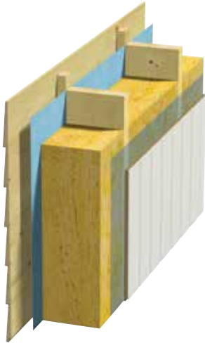
Fig. 5 Exterior wall Timber upright, foil wind barrier.
