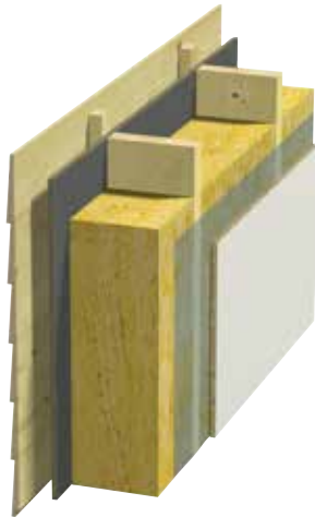
Fig. 8 Exterior wall Timber upright, wind barrier, 12 mm wood fibre-board.
