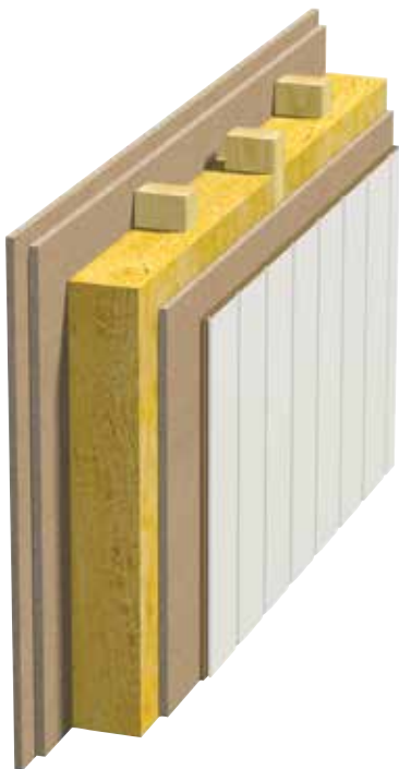
Fig. 3 Interior wall Displaced timber upright on timber sill. Two board layers.
