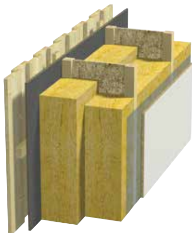
Fig. 3 Masonite upright, wind barrier, 12 mm wood fibreboard.
