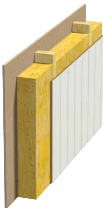
Fig. 1 Interior wall Continuous timber upright. One layer of board.
