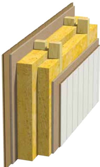
Fig. 4 Interior wall Double timber upright. Two board layers.
