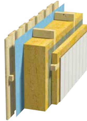
Fig. 6 Exterior wall Timber upright, foil wind barrier with interior crosser liner.
