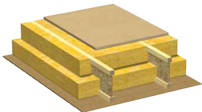
Fig. 1 Beam structure Masonite floor beams, fully insulated with ceiling attached directly to the floor beams 1).
