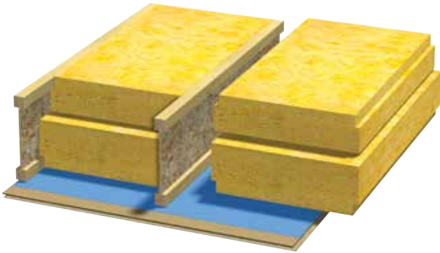
Fig. 5 Roof Ceiling against cold attic.
