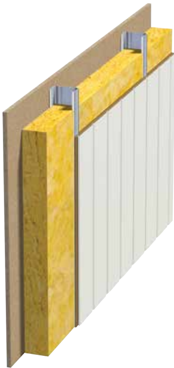
Fig. 5 Interior wall Continuous steel upright with one board layer.
