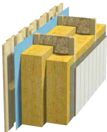
Fig. 1 Exterior wall Masonite upright. Foil wind barrier.
