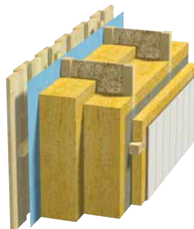
Fig. 2 Exterior wall Masonite upright, foil wind barrier with interior crosser liner.
