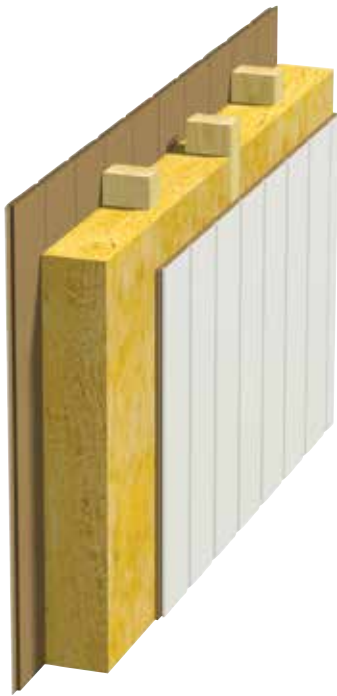
Fig. 2 Interior wall Displaced timber upright on timber sill. Two board layers.
