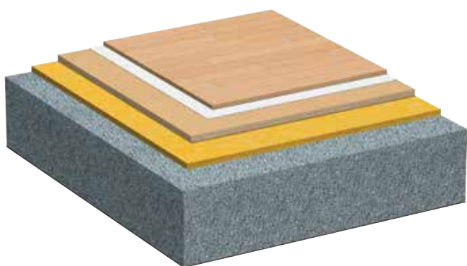
Fig. 1 Covering. Floating floor on lightweight clinker.
