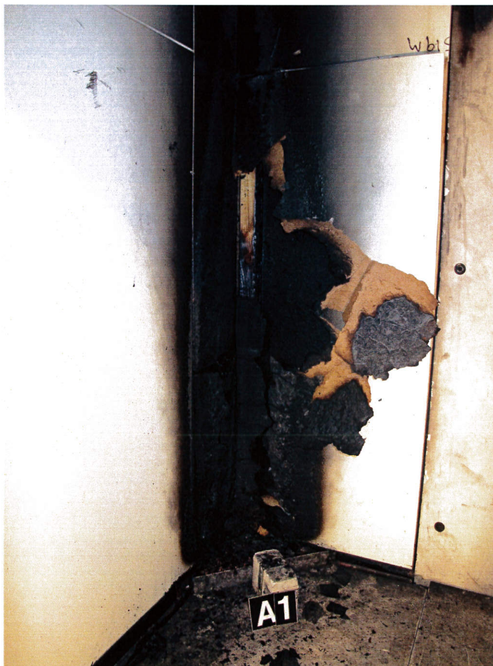
Photo no 3 After test “Huntonit Brannit with Palett”
